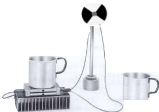
Fig. 8: Experiment to demonstrate the symmetry of the Seebeck effect
