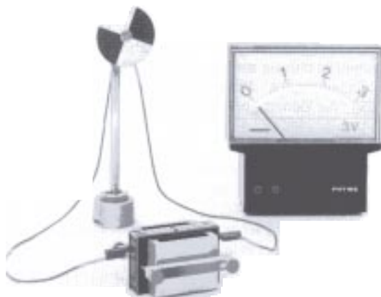
Fig. 7: Thermal energy is transformed into electrical energy
